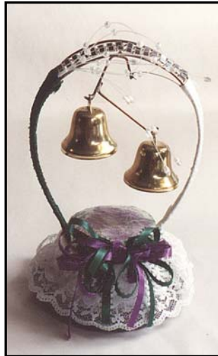
Solar-powered Wedding Cake centerpiece. Powered by a twin-string of photodiodes producing 9 volts at 1.5mA, this device swung the bells to and fro every 6 minutes.
