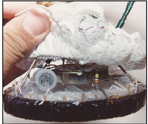
Solar-powered Wedding Cake centerpiece. Powered by a twin-string of photodiodes producing 9 volts at 1.5mA, this device swung the bells to and fro every 6 minutes.
